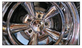
**Step 3:** This is how the Tower looks after you slide your Supreme wheel over it. The studs will travel through the Tower and your wheel. Install your lug nuts and tighten them to the correct settings. Supreme Wheel Spinner Kit Installation Instructions
