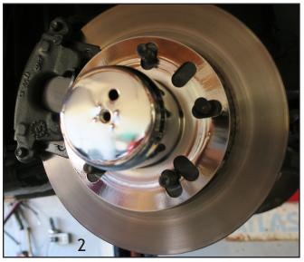
**Step 2:** Shown is a disc brake set-up on the front of a car. Simply slide the Tower onto the matching studs. The Tower should sit flat on your brake drum or disc brake mounting surface. Your studs will align with the corresponding holes in the Tower. Next, you will install your Supreme wheel on top of the Tower.
