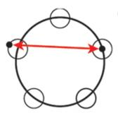
A Begin by measuring your **bolt pattern**. Note how you measure from the center of one hole to the outside or furthest edge of the hole diagonally across from it.
