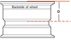
Side view of wheel with back side up. Lay your wheel down to measure. Measure with a straight edge across the back lip of the wheel.
